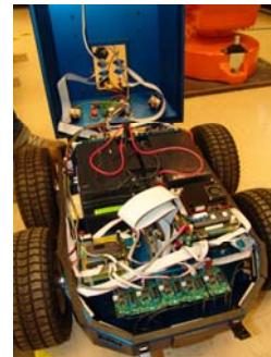
Figure 1.0 Robot electronic components inside the chassis
