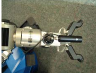
Figure 6.1 Camera position on top of the Harmonic arm
