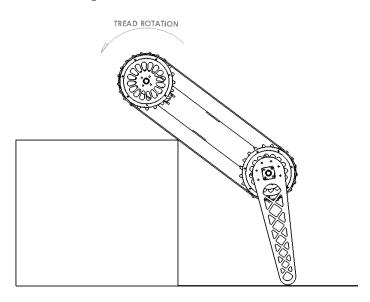
Step 4: The robot is now moving forward and the arms are only stabilizing the robot from flipping over. If the robot does fall over backwards or the object is too tall, the arms can simply flip the robot upright.
