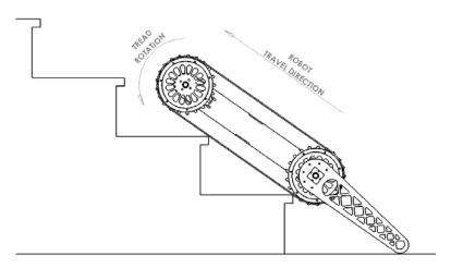
The robot can now climb the stairs without flipping over backwards.
