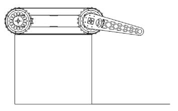
Step 5: The robot has now climbed on top of the object. The multipurpose arms can now be rotated back into a position that the next object requires.
