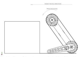
Step 1: The arms have lifted the front of the robot up to the height of the object it is about to climb. The rounded front ends of the arms allow the robot to still travel in a forward motion until it reaches the object.
