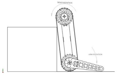
Step 3: The arms and treads continue to move in the same direction as in step 2. The arms are strong enough to lift the entire weight of the robot off the ground.
