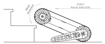
Step 1: The robot has lifted the front end up high enough to clear the first step. The robot then drives forward just far enough to rest on the top of the first step.
