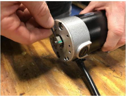
6. Once the hex bolt is removed reattach brake onto main motor, then reattach the cap.
