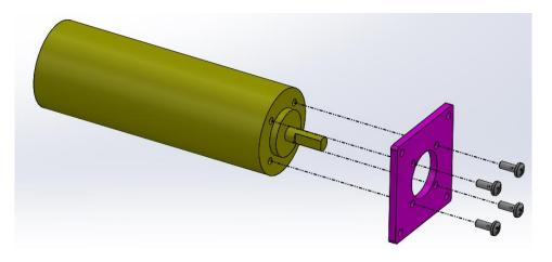
2. Use the included #4-40 hardware and plastic spacers to mount the motor plate to the motor tube.
