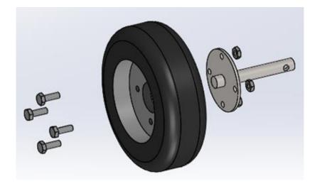
6. Mount wheel assembly to motor assembly. Slide a lock collar over the shaft before installation. Insert wheel shaft through ball bearing. Before sliding the wheel shaft onto the motor, slide on a second lock collar. Align the set screw holes on the wheel shaft and the lock collar to the flat spot on the motor shaft. Firmly press the wheel shaft inward against the motor and secure the set screw with Loctite.
