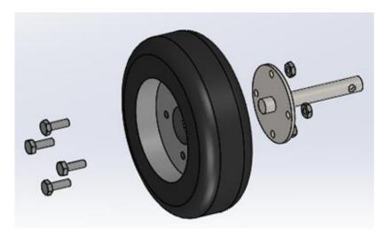
5. Mount wheel assembly to motor assembly. Slide a lock collar over the shaft before installation. Insert wheel shaft through ball bearing. Before sliding the wheel shaft onto the motor, slide on a second lock collar. Align the set screw holes on the wheel shaft and the lock collar to the flat spot on the motor shaft. Firmly press the wheel shaft inward against the motor and secure the set screw with Loctite.
