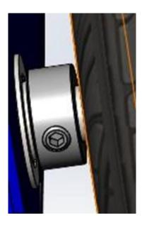
7. Install standoffs onto main chassis with provided hardware. Use Loctite to secure screw to standoff on the chassis.
