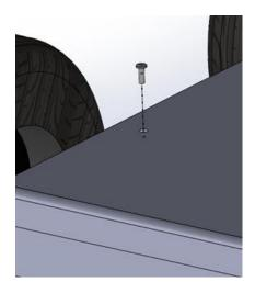
9. There are a variety of options for purchase when selecting your robot. If you have selected additional items that require additional mechanical assembly, please be safe doing so. Hardware will be provided to mount those items. Check both sides of the surface before beginning to work and hold the part in place to ensure that it will not interfere with any of the other components before drilling. Mark your holes with a pen or pencil and pilot drill holes with a 3/32" drill bit.
