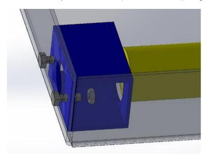
3. Insert ball bearing to support the wheel shaft. Additional filling may be needed to fit bearing through chassis into motor tube. Test fit each bearing to find the bearing that works best for each bearing hole.
