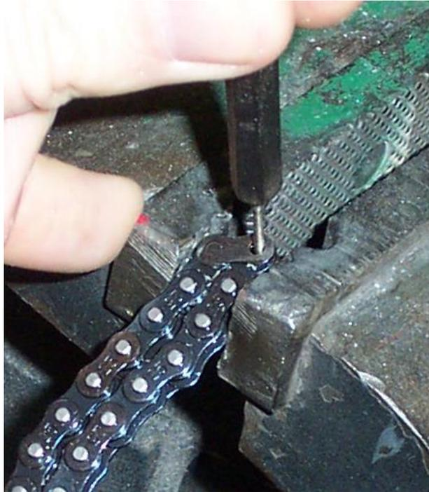
9. Install the master link as shown in the figure below **Error! Reference source not found.** and tension chain by sliding the motor away from the axle. The chain should be tight enough so there isn't much slack but loose enough so that it isn't adding extra strain on the motor shaft. Listen when running the robot to notice if there is an uneven sound coming from the motor. If so, the chain is probably too tight.
