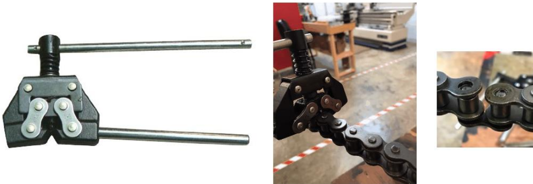
Figure 6: Chain breaker tool
