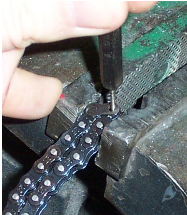
Figure 9: Chain Link removal
