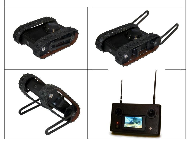
SuperDroid Robots Compact MLT Tactical Surveillance Robot. It weighs less than 8lbs and is drop resistant up to 10 feet. The treaded design and rear flipper arms allow this robot to climb many obstacles other throwable robots can't touch!
