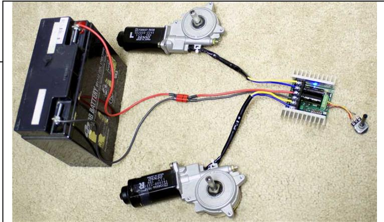
The 5V terminal can be used to power small loads, like a potentiometer or a radio receiver. The 0V signal must be connected to the ground of the device generating the input signal.
