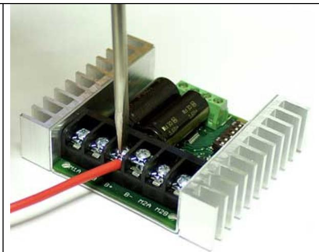
**Step 4:** Turn the top screw clockwise until you encounter resistance, then tighten the screw firmly. Pull on the wire gently to ensure that it is secured.
