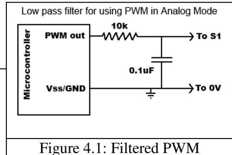
Figure 4.1: Filtered PWM
