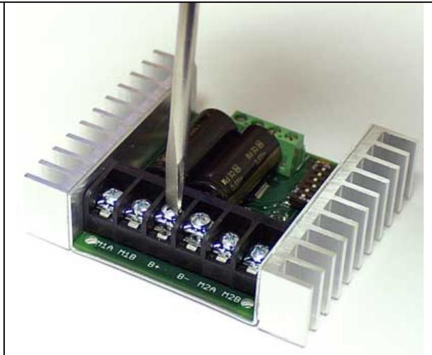
**Step 2:** With a large screwdriver, turn the top screw counter-clockwise until it stops gently.
