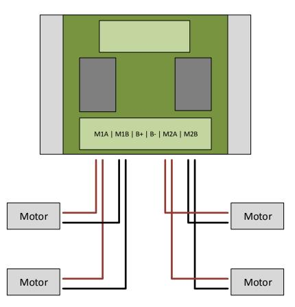
Note: If running multiple motors, parallel motor wires at the motor controller as shown.
