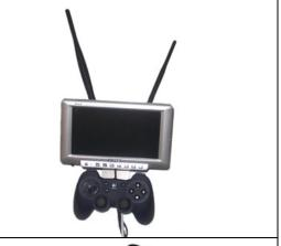
WiFi Controller Option: This option uses a WiFi connection similar to the one above, but utilizes a Ultra-Compact PC. The Color touch screen LCD can be used to control the robot and view the IP camera(s). The PC is mounted in a custom bracket with a gamepad controller mounted to it. We provide a program so all the driving and control of the robot is done using the using the robot control program using the game pad controller and touch screen LCD.
