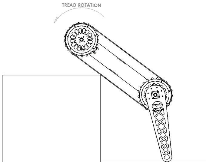
Step 4: The robot is now moving forward and the arms are only stabilizing the robot from flipping over. If the robot does fall over backwards or the object is too tall, the arms can simply flip the robot upright.
