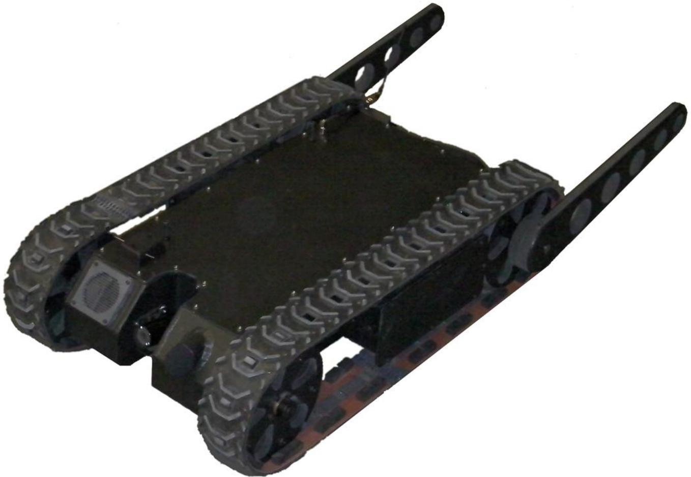
The LT2-F was qualified during a series of NIST tests. The robot package includes a complete robot including the, a selection of a custom remote, and selection of a front tilt camera, and battery charging station. The LT2-F is capable of climbing household stairs and obstacles, very maneuverable, able to inspect under vehicles and houses. It can also be equipped with 2 way audio for hostage negotiation.
