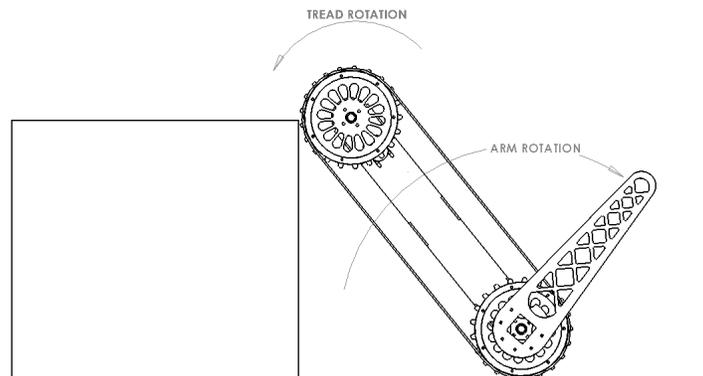
Step 2: The robot is now resting on the object while the arms are rotated backwards. The treads are moving slowly forward at this time.
