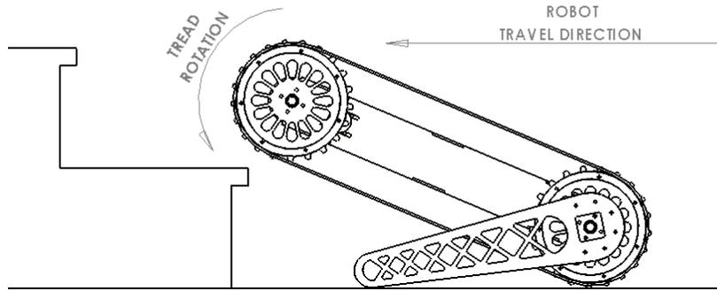
Step 1: The robot has lifted the front end up high enough to clear the first step. The robot then drives forward just far enough to rest on the top of the first step.
