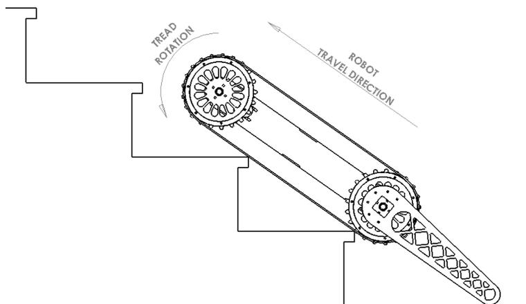
The robot can now climb the stairs without flipping over backwards.
