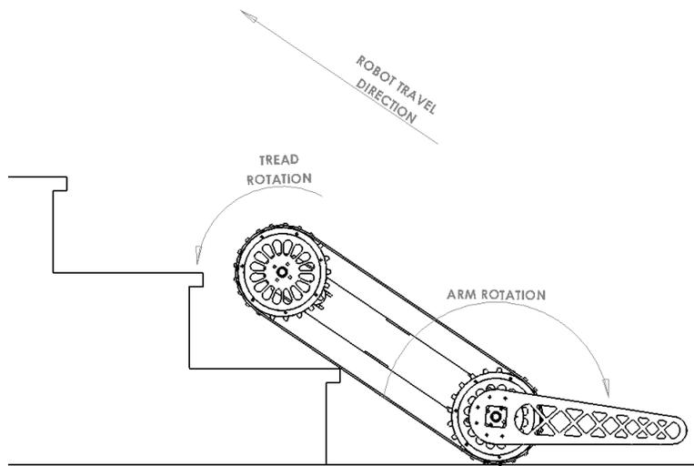
Step 2: The arms are rotated in the direction of the arrow shown. Once the arms are about to reach the ground the robot can drive forward. The arms act as a stabilizer bar that prevents it from turning over.
