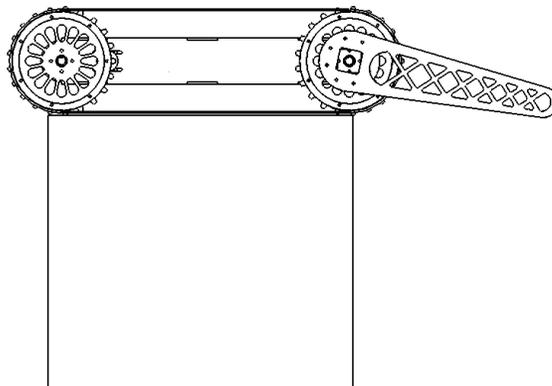
Step 5: The robot has now climbed on top of the object. The multipurpose arms can now be rotated back into a position that the next object requires.
