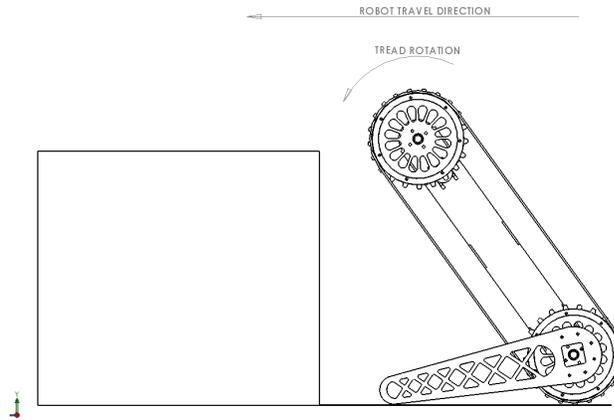
Step 1: The arms have lifted the front of the robot up to the height of the object it is about to climb. The rounded front ends of the arms allow the robot to still travel in a forward motion until it reaches the object.
