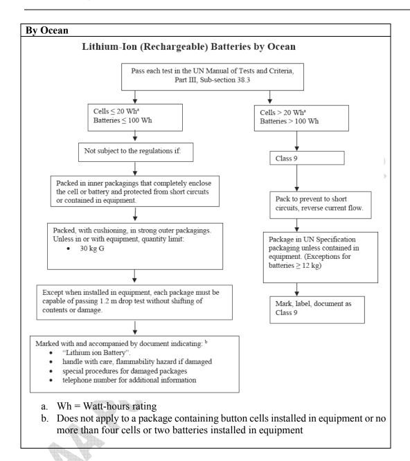
Separate Li-ion batteries when shipping to prevent short-circuiting. They should be packed in strong packaging for support during transport. In the case of transportation, confirm no leakage and no overspill from a container. Take in a cargo of them without falling, dropping and breakage. Prevent collapse of cargo piles and wet by rain. The container must be handled carefully. Do not give shocks that result in a mark of hitting on a cell. Please refer to Section 7-HANDLING AND STORAGE also.
